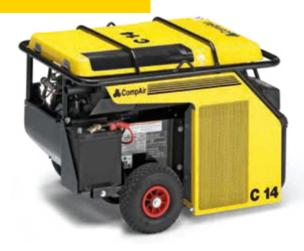
C10-12 to C14 is a powerful alternative to electrical tools. Small, compact and lightweight, at only 165kg weight with 1.0 to 1.4 m<sup>3</sup>/min at 7 to 12 bar. Perfect for a widerange of repair and installation jobs.
