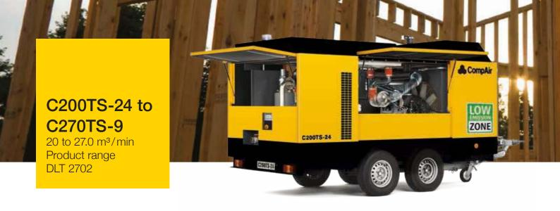
The TurboScrew compressors with their unique patented bi-turbo technology provide class-leading diesel efficiency, the lowest weight of 3,500kg and super-clean performance in accordance with directive 97/68/EC Stage 4 final. The new range has been equipped with an award winning SCRT® – Selective Catalytic Reduction Technology system which is capable of removing almost all nitrogen oxide emissions from diesel exhaust gases.
